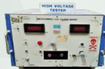
High Voltage Tester Range upto 4KV
