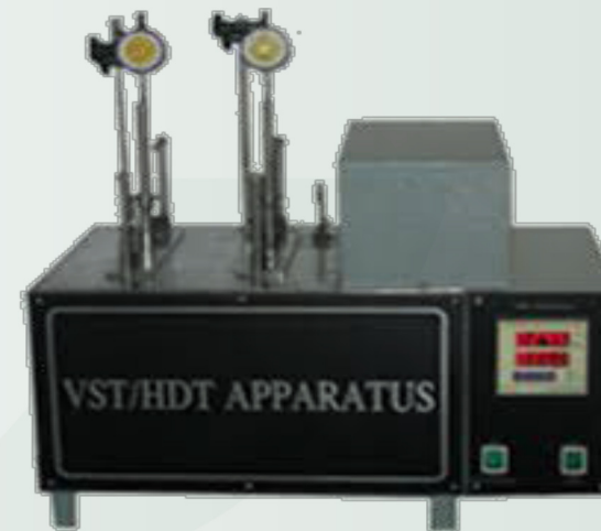
Heat Distortion Temperature Apparatus (HDT)
