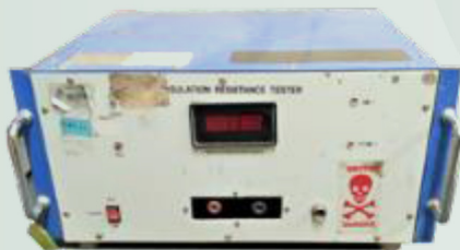
Insulation Resistance Tester Range 50k to 1G Ohm
